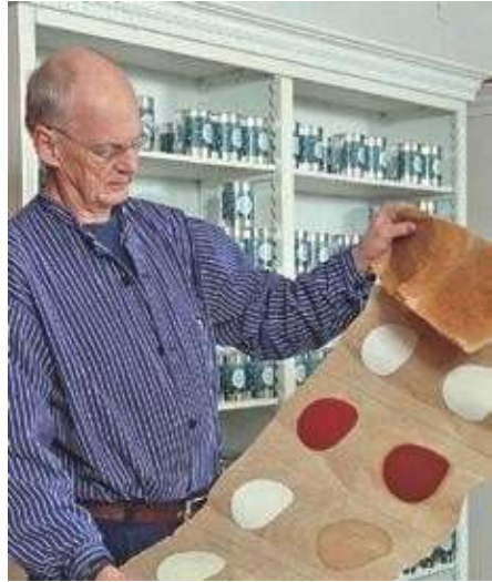
Paint on absorbent surfaces! One simple test to check the penetration and protective abilities of the paint/oil.
